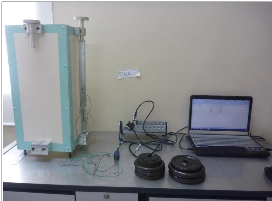
Figure 5.5: The connection of Data Logger to the laptop and test rig
