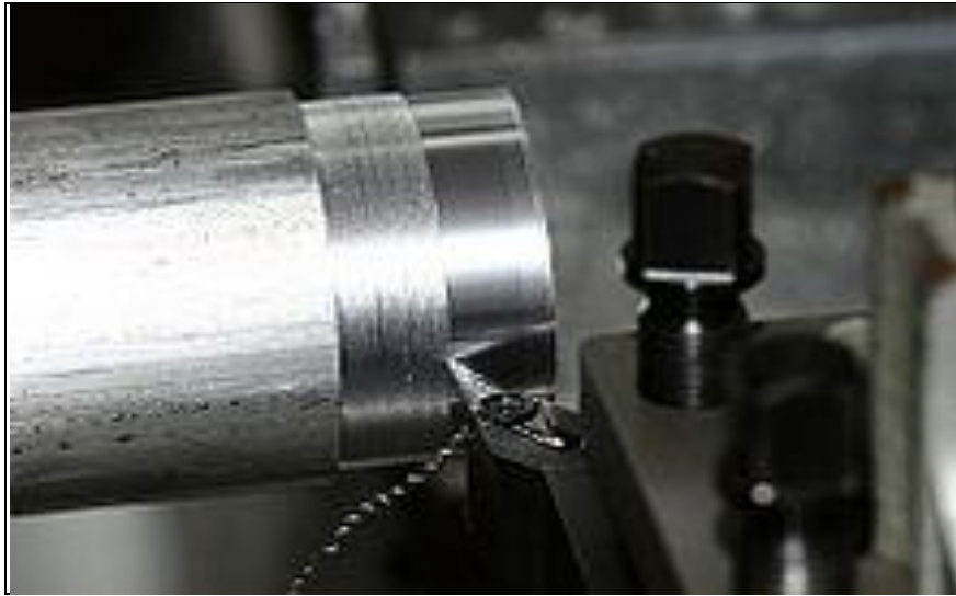
Figure 4.29: Finish turning step
