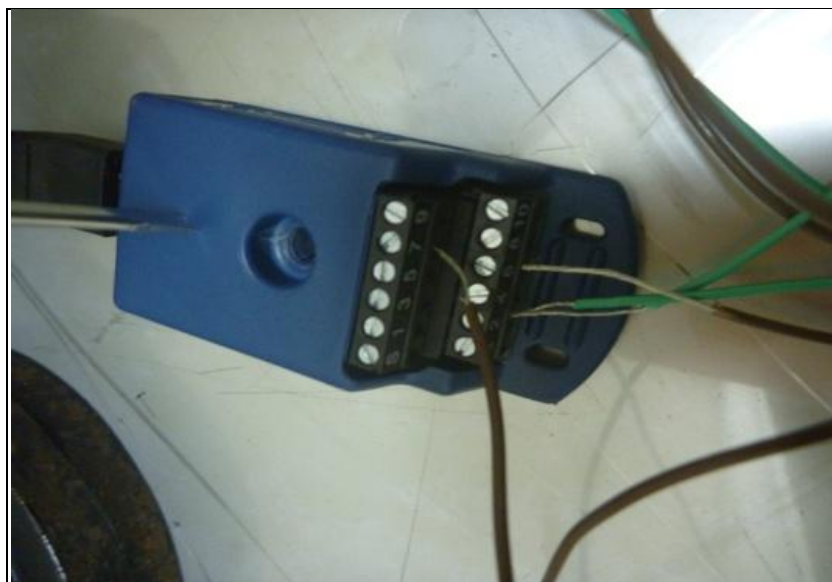
Figure 5.3: How Strain Gauge connects with Data Logger
