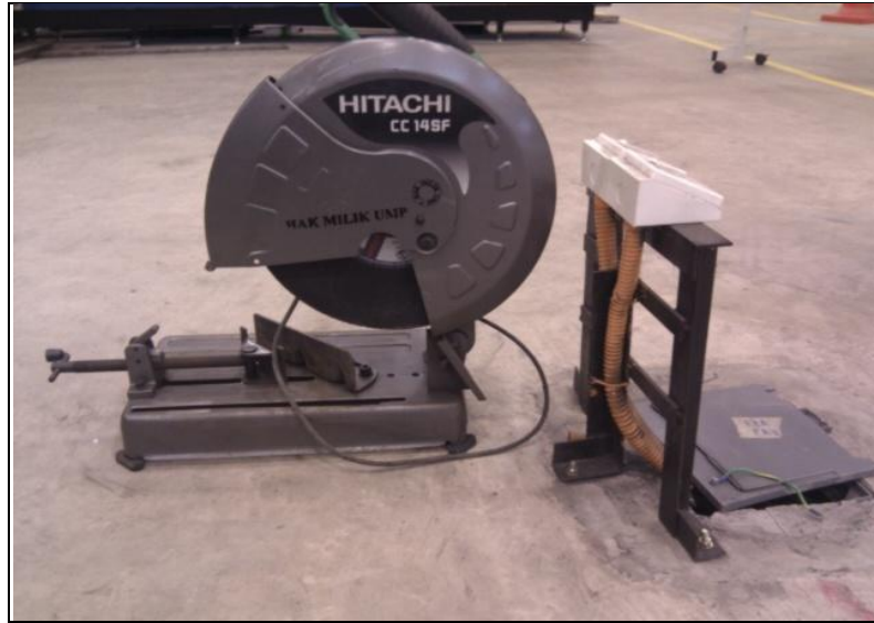
Figure 3.8: Examples of cutting disk (Model HITACHI SS 14SF)
