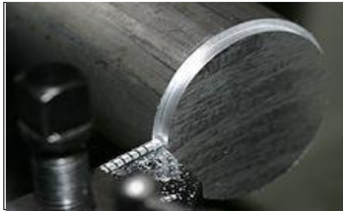
Figure 4.27: roughing or rough turning step
