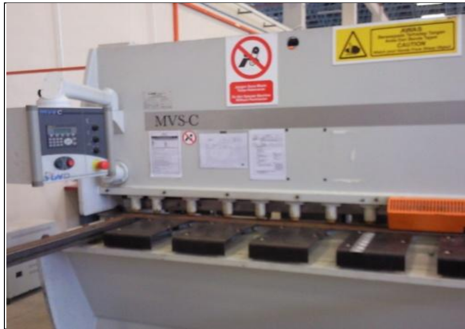
Figure 3.10: MVS-C shear cutting machine
