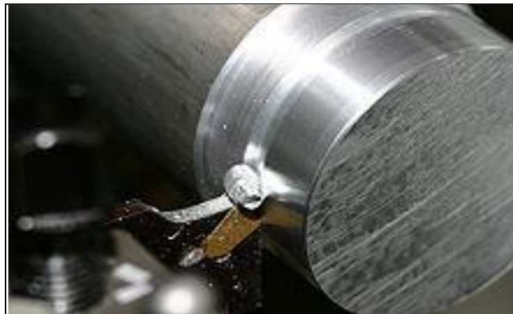
Figure 4.28: Parting aluminium step
