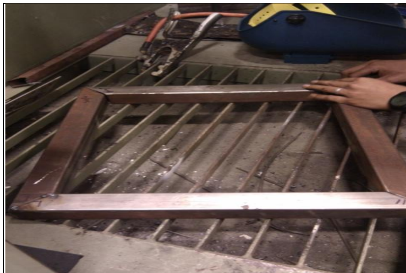
Figure 3.4: Example on welding process on hollow iron/steel
