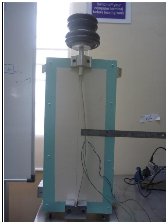
Figure 5.1: Strain gauge test using DASY Lab software
