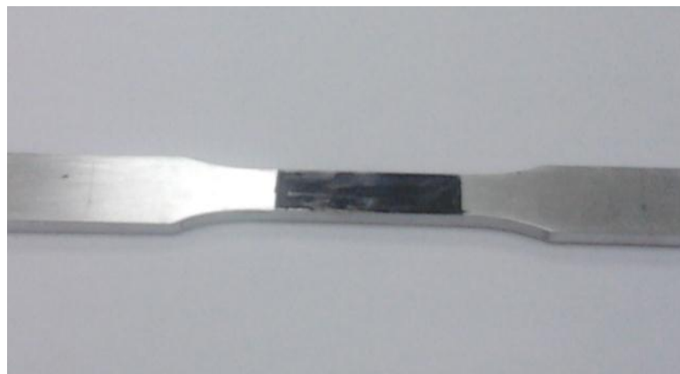
Figure 3.11: The marking zone for aluminum specimen
