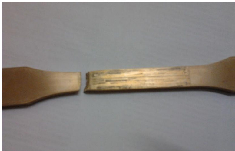
Figure 3.14: The specimen condition after break for brass
