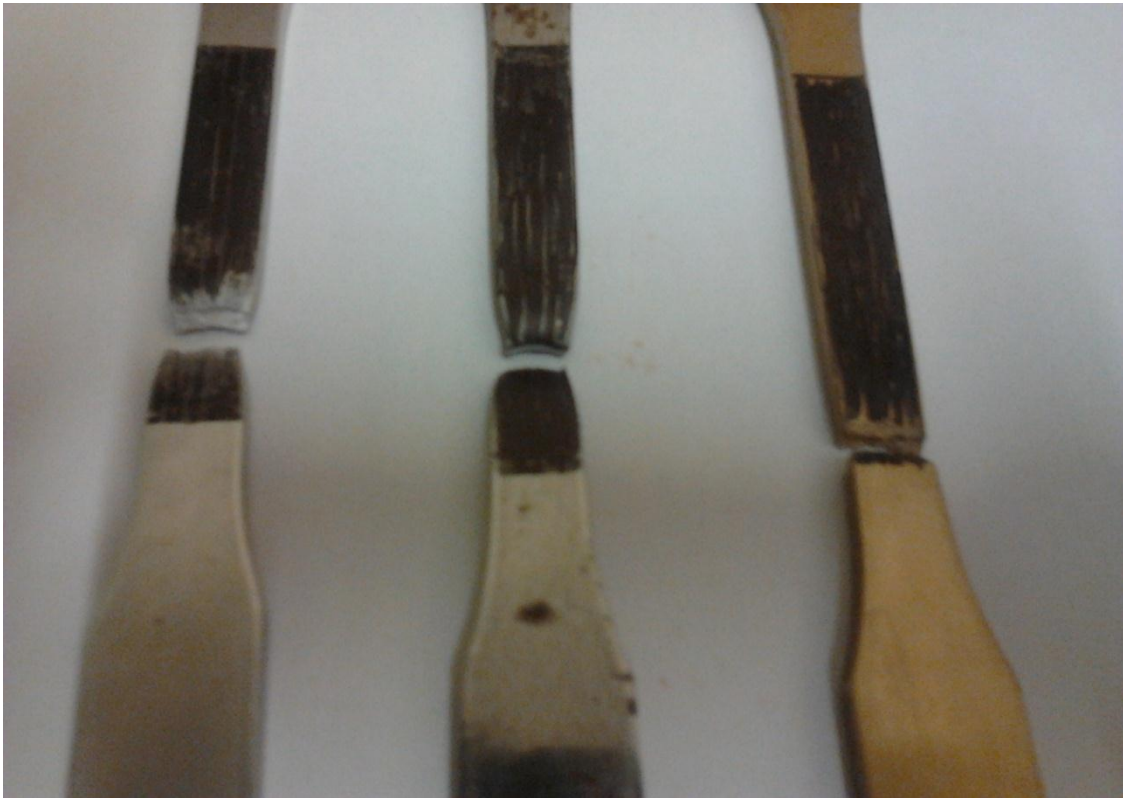
Figure 4.7: Failed specimen for all material. From left are aluminum, mild steel and brass.
