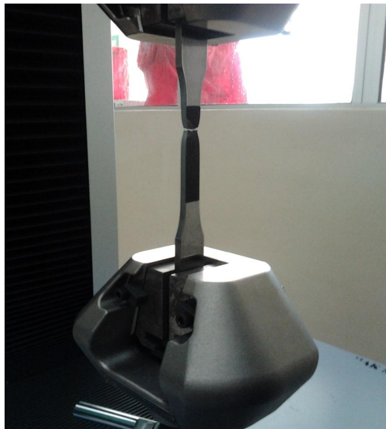
Figure 3.16: The specimen break during tensile test
