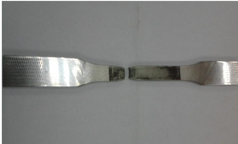
Figure 3.15: The specimen condition after break for mild steel
