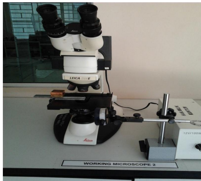
Figure 3.19: The measurement process by using microscope and dial gauge
