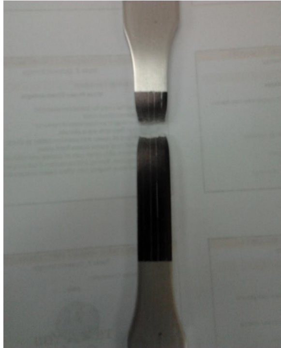
Figure 3.13: The specimen condition after break for aluminum
