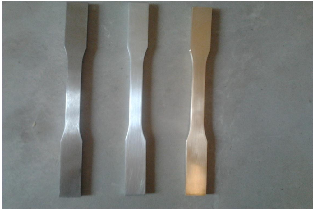
Figure 3.8: The surface finish after polishing using sandpaper
