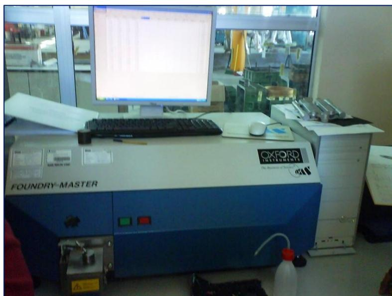
**Figure 3.5:** Spark emission spectrometer
