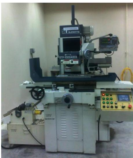
**Figure 3.8:** Surface grinding machine
