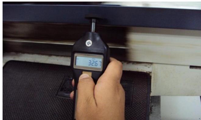
**Figure 3.10:** Calibration of table speed
