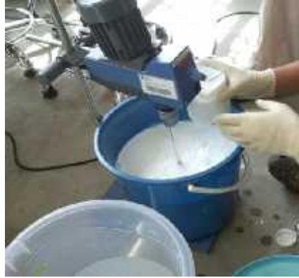
Figure 3.3: Nanofluid Prepared by Two Step Method
