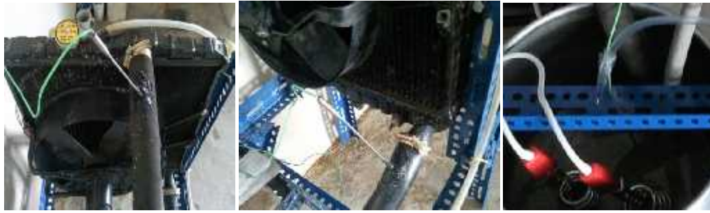
Figure 3.9: Thermocouples Placed at Three Locations
