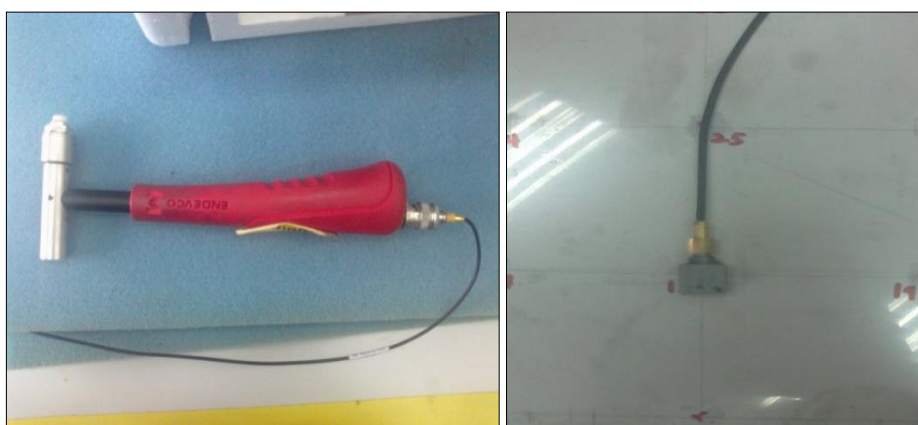
Figure 3.3: Transducer used for excitation (left) and response measurement (right).
