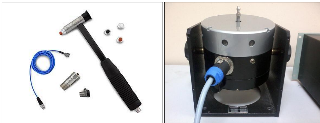
Figure 2.3: Hammer and Shaker Excitation
