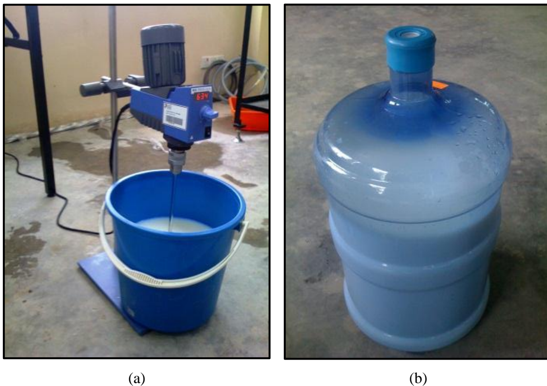
Figure 3.5: (a) Stirring process; (b) The prepared TiO 2 nanofluid
