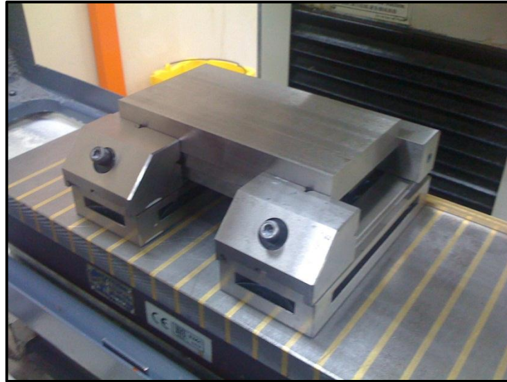
Figure 3.10: The steel clampers used to clamp the work piece during the experiment
