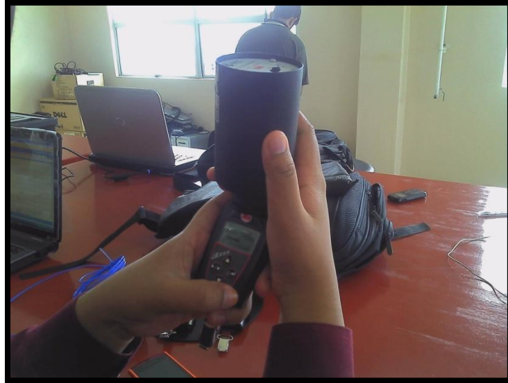
Figure 3.10: One of the calibration process, calibrating dosimeter before data measurement process.
