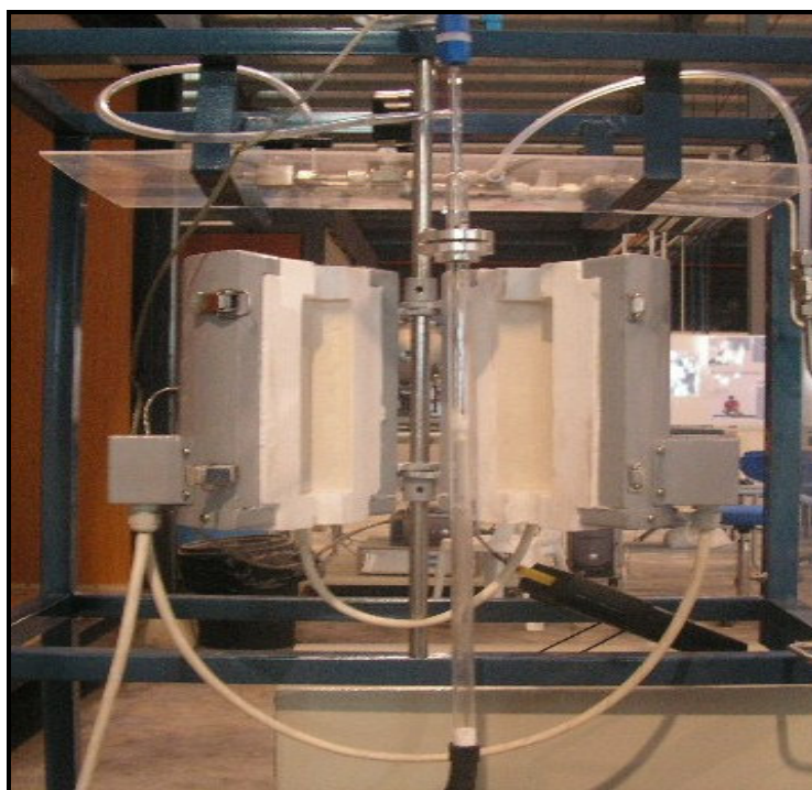
Figure B.7: Picture of electrical furnace that used for catalyst treatment.
