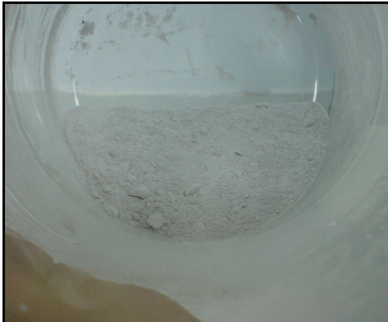
Figure B.5: Picture of sample after drying in oven at 120°C for over night.
