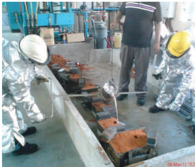
Figure 3.7: Molten metal was pouring to the mold
