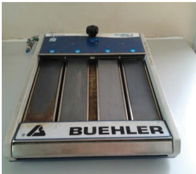
Figure 3.12: Buehler HandiMet 2, Roll Grinder
