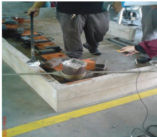
Figure 3.5: Checking the temperature before pouring to the mold
