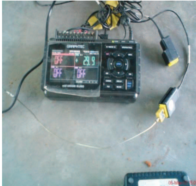
Figure 3.6: Thermocouple for checking the molten metal temperature
