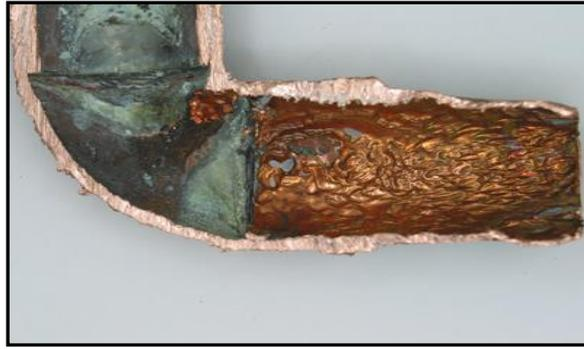
**Figure 2.7:** Impingement failure of an elbow that was part of a steam condensate line.
