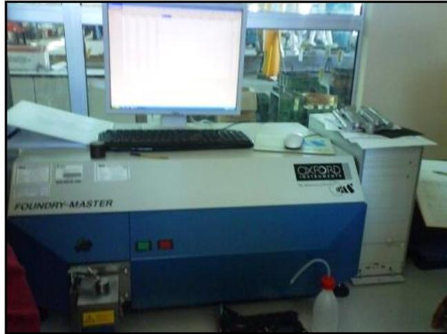
**Figure 3.4:** Spark emission spectrometer
