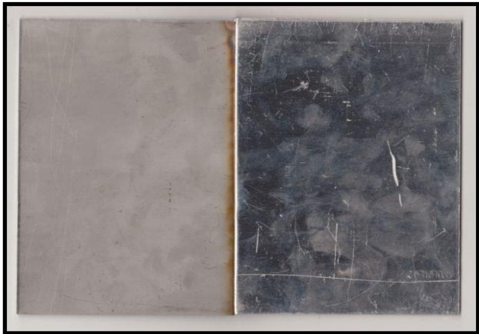
Figure 4.2: Back view of joining plate by MIG welding
