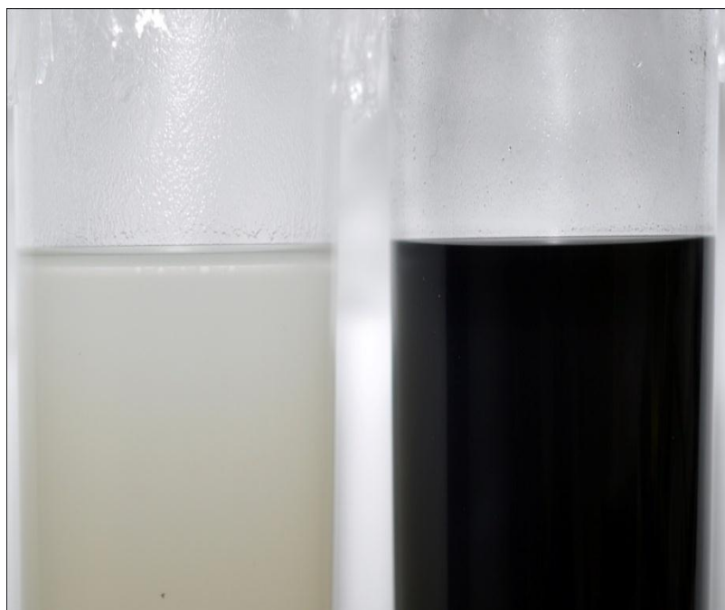
Figure 4.8: Dispersion stability after 3 hour stir. (25/4/2012 01:36 PM)
