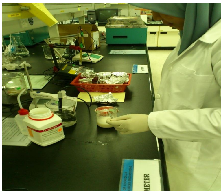
Figure 3.8: Neutralization process by using calcium hydroxide
