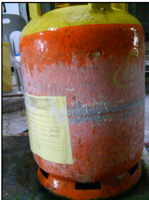
Figure 4.3: Sweating of LPG Tank
