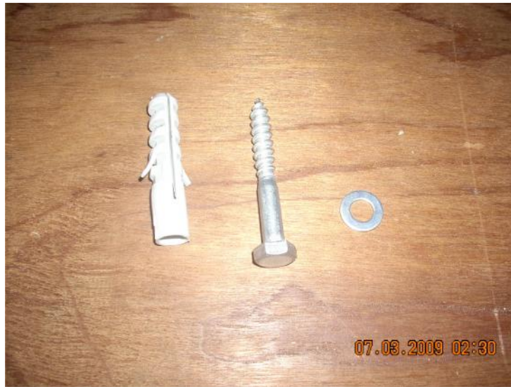
Picture 5 : Lag bolt, concrete anchor and lag washer
