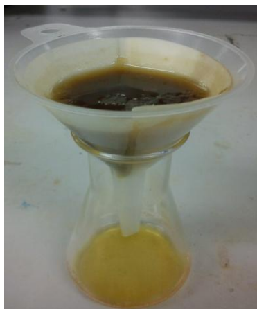
Figure 4.4 Filtration of Cracked Oil
