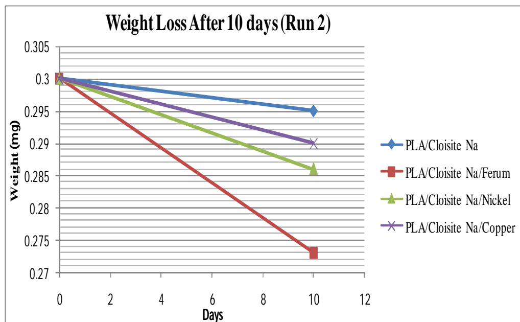
Figure 4.24: Weight Loss after 10 days (Run 2)
