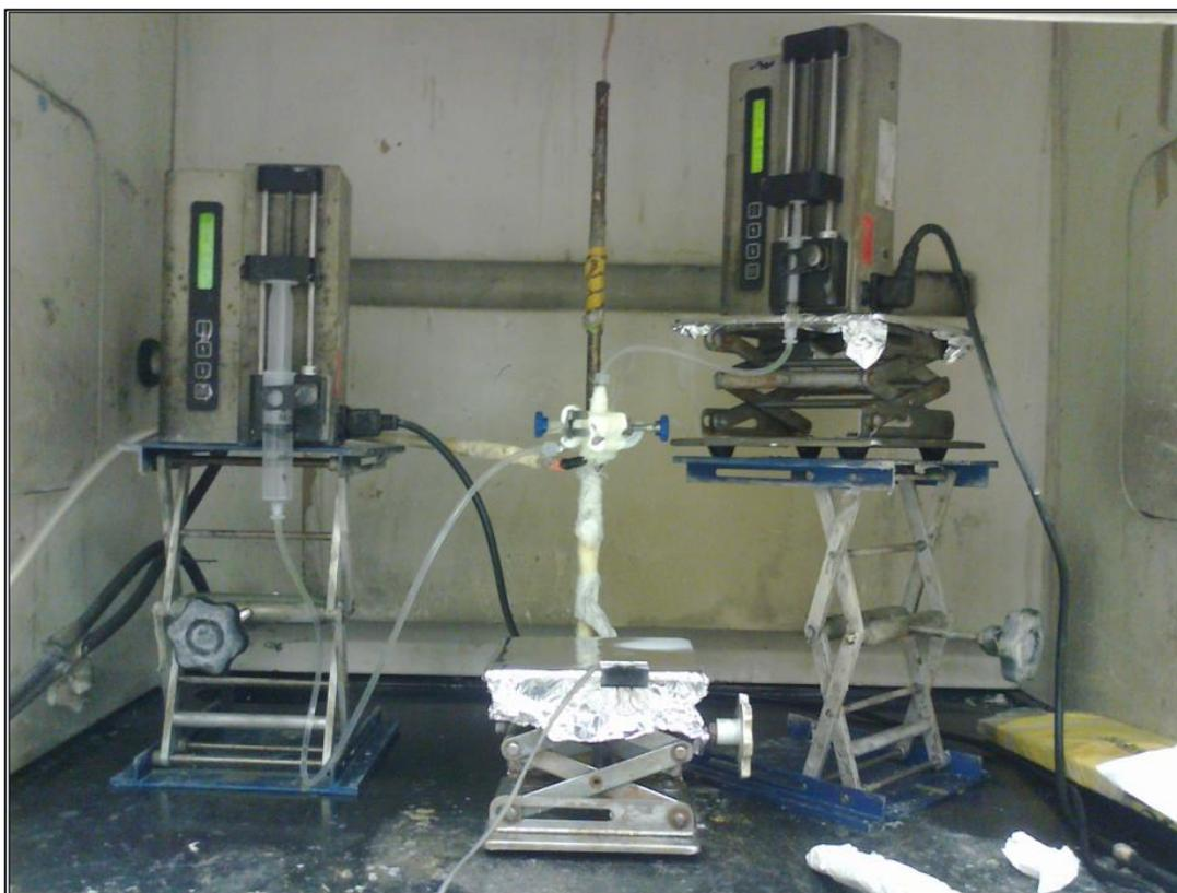
**Figure 3.3:** Co-axial electrospinning setup. Co-axial nozzle configuration was used with 2 different sizes of needles were attached to it and the flow rates of the solutions were controlled by the syringe pumps.
