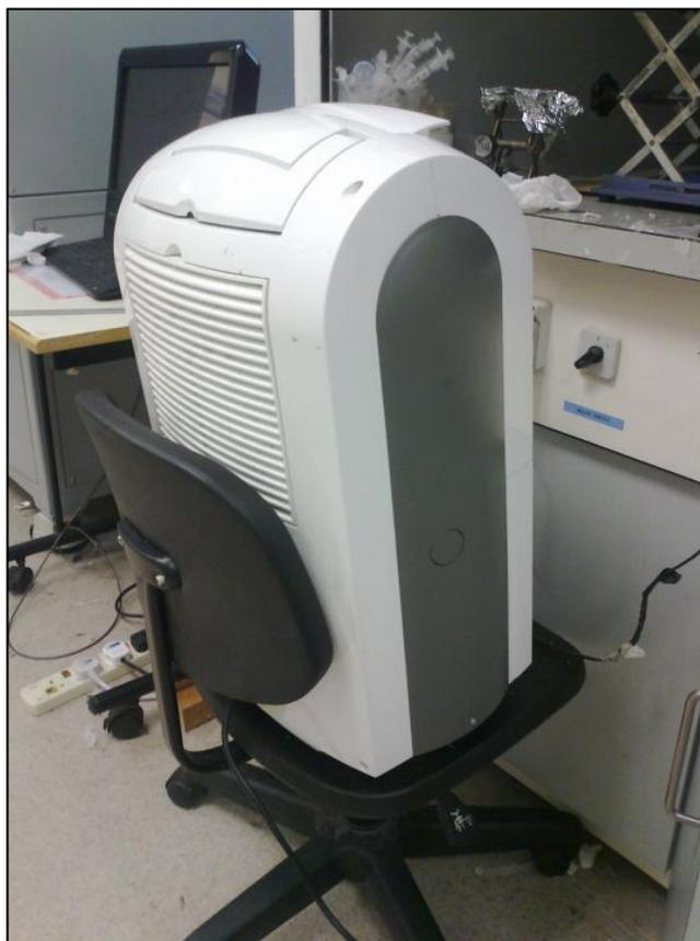
**Figure 3.6:** Humidifier to control the humidity inside the electrospinning chamber
