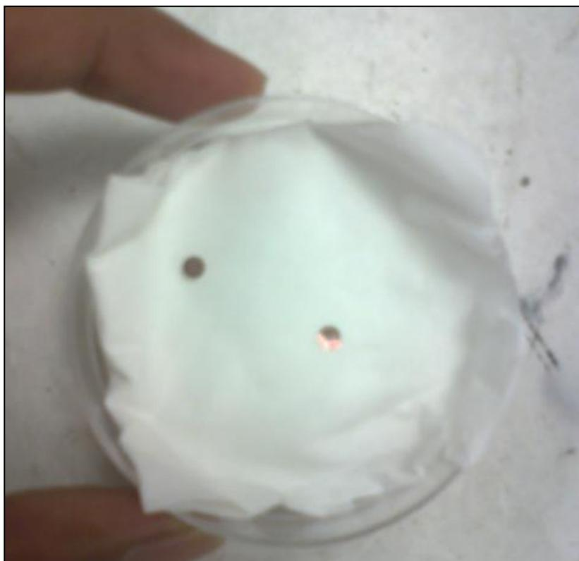
**Figure 3.7:** Carbon grid preparation for morphological analysis using TEM
