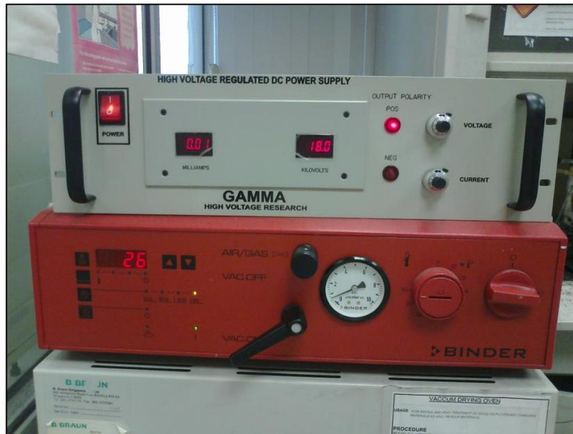
**Figure 3.4:** High voltage power generator to supply positive direct current to the electrospinning setup
