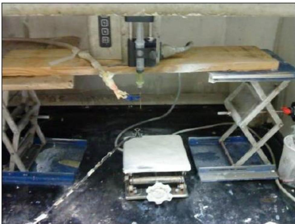
**Figure 3.2:** Mono-axial electrospinning setup
