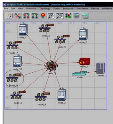
FIGURE 4. 3 Star topology Example
