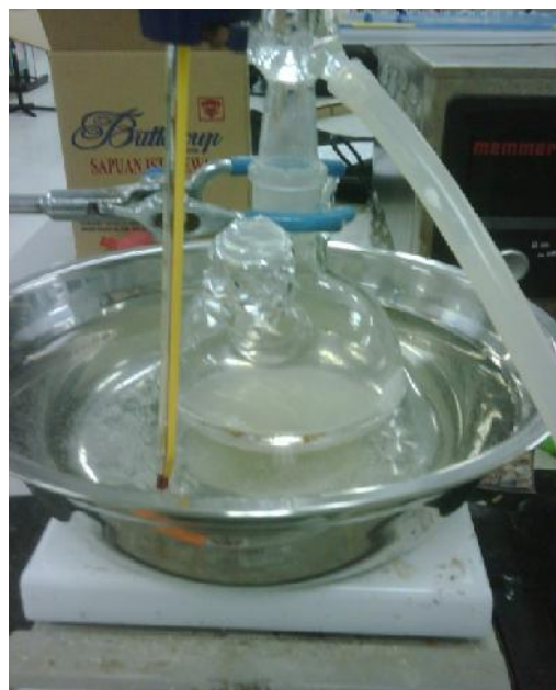
Figure B.2: Esterification Reaction with Batch Reactor
