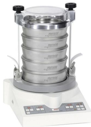
Figure 3.3 – Laboratory sieve shaker
