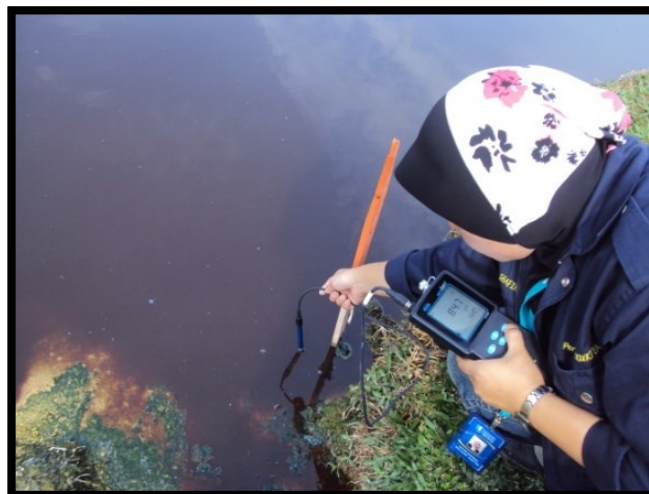
Figure 3.0: Checking pH and temperature parameter at the final effluent discharge.
