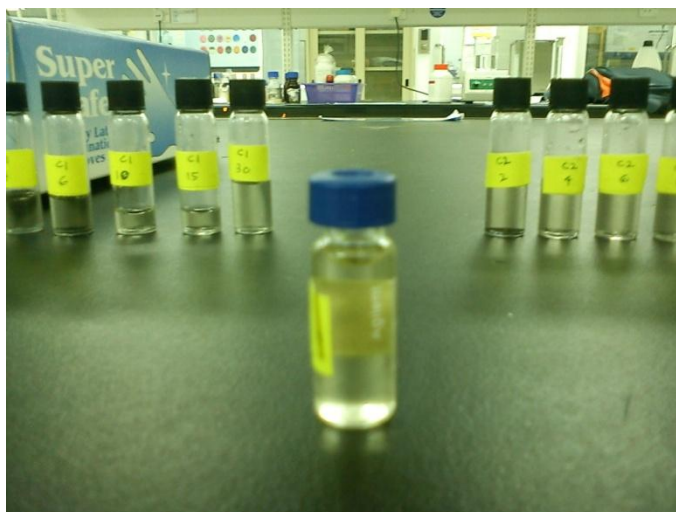
Figure 3.5: Vial fill-up with AA sample for HPLC Analysis
