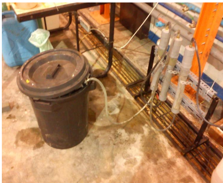
Figure 3.2: Overview of Continuous Fixed-Bed Adsorption System
