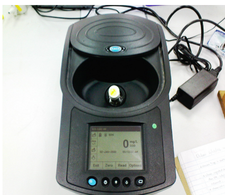
Appendix A.4: DR 2800 Spectrophotometer (HATCH)
