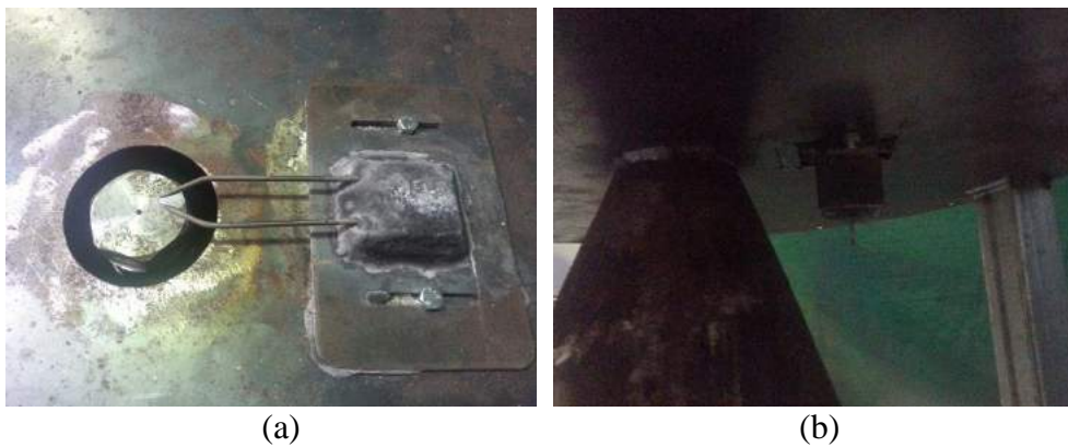
Figure 11. Ignition system: (a) ignition lead top view (inside the burner); (b) bottom view (outside the burner)
