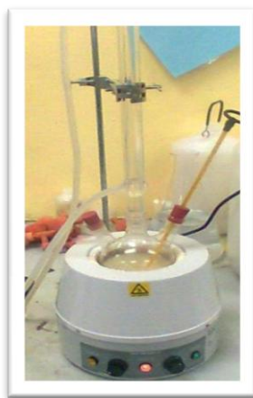
Figure A.1: Biodiesel production using heating mantle
