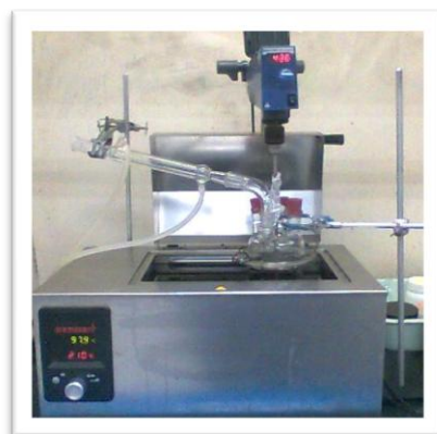
Figure A.2: Biodiesel production using oil bath
