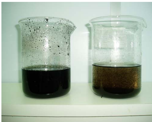
Figure 4.1: Samples of EFB after the two-stage hydrolysis at 80°C using water bath for two hours
