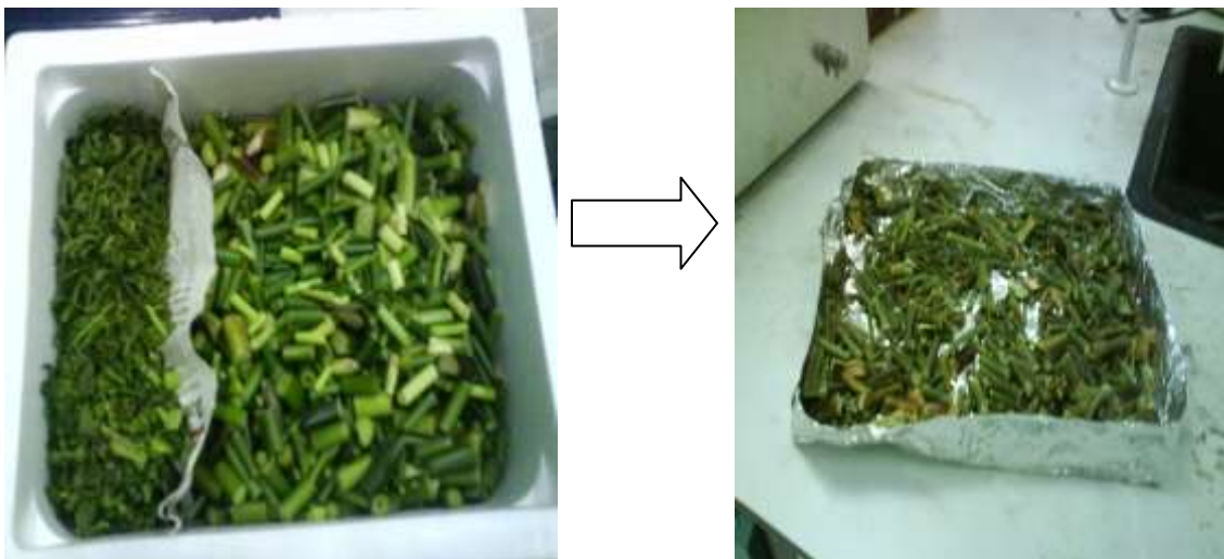
Figure A4: Water hyacinth before and after drying in the oven over 24-72 hours
