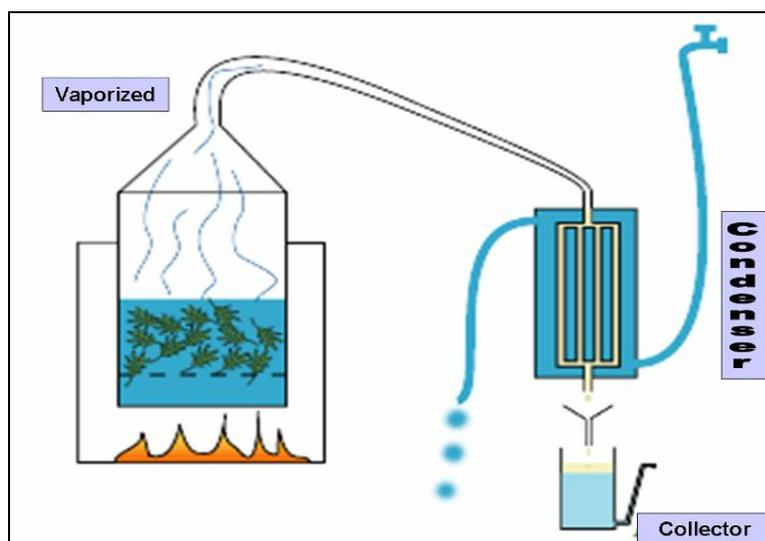
**Figure 1.2: Simple Hydro Distillation Concept**
