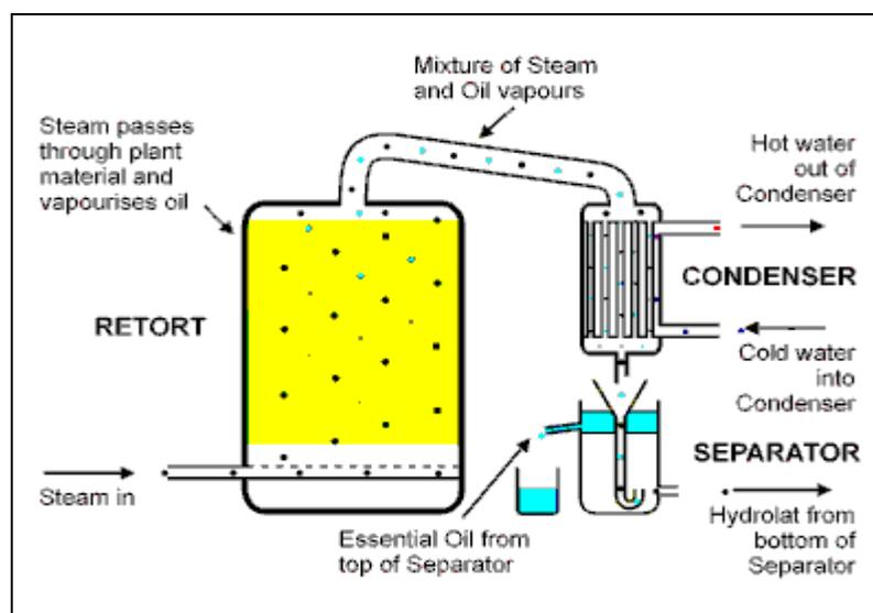
**Figure 1.3: Simple Steam Distillation Unit**
