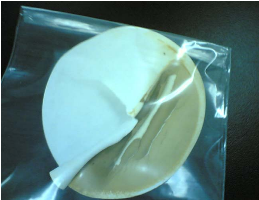
Figure B-4: Colloidal solids extracted from alum sludge
