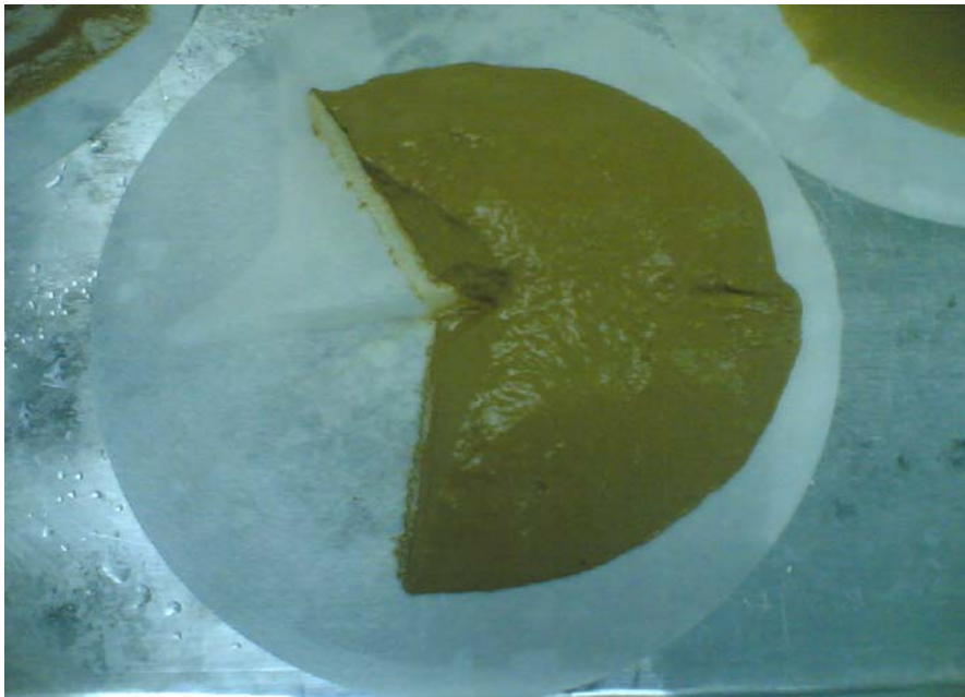
Figure B-2: Alum sludge sample proven for gelatinous property
