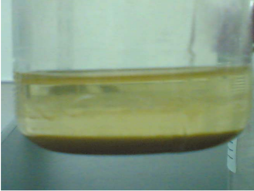
Figure B-3: Process of settling/ precipitate of alum sludge sample
