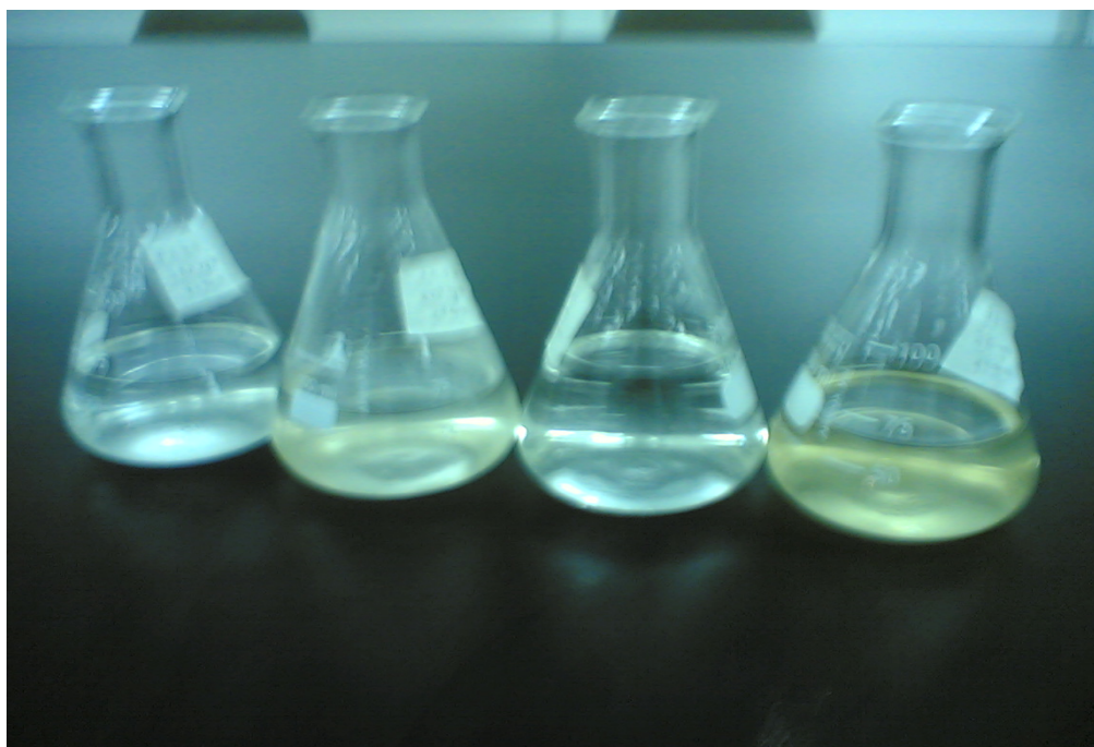
Figure B-6: Aluminium Sulphate recovered from Alum Sludge
