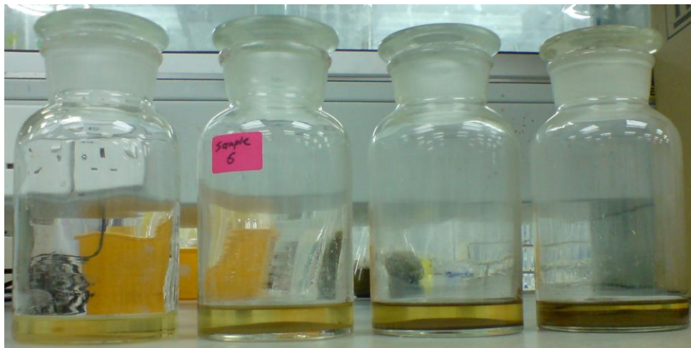
Figure 4.2: From the left, isooctane samples for 600 rpm, 780 rpm, 960 rpm and 1140 rpm of Zeolite catalyst.
