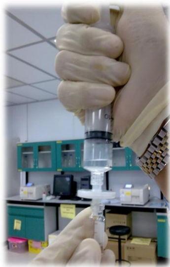
Figure B.7: Syringe 10ml and 0.2µm syringe filter
