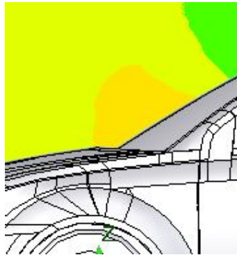
Figure 4.7: Pressure Distribution at Windshield and Cowl
