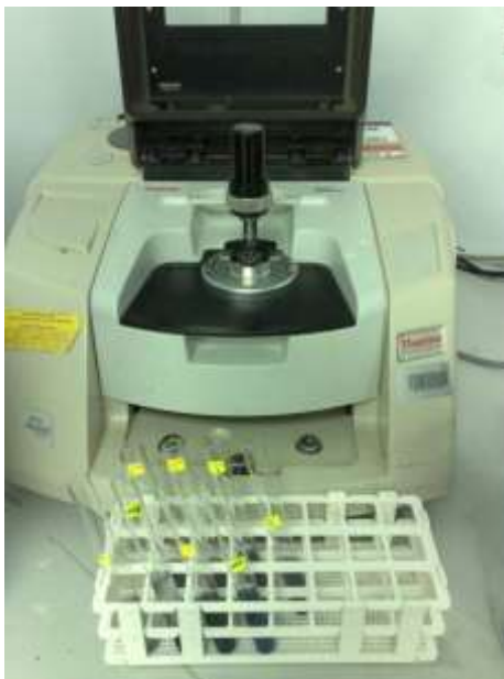
Figure 3-14 Sample characterization using FTIR
