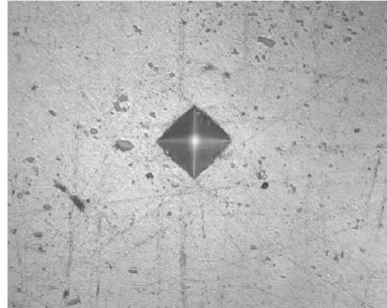
**Figure 4b Indentation sample of the Diamond Indenter**
