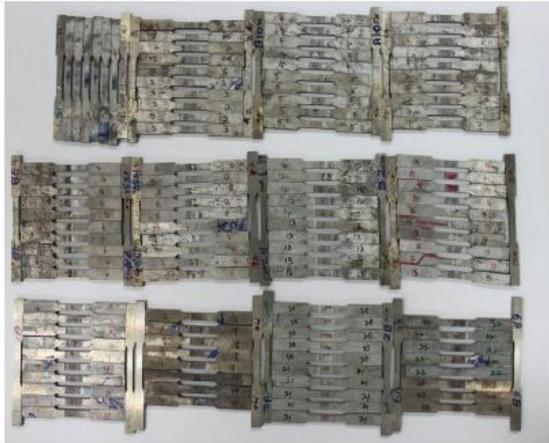
**Figure 3a Samples Cut from EDM**
