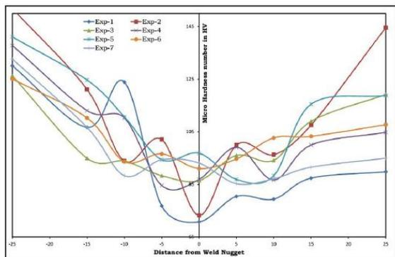
Figure 6b Micro hardness perpendicular to the weld line from Hardness Test
