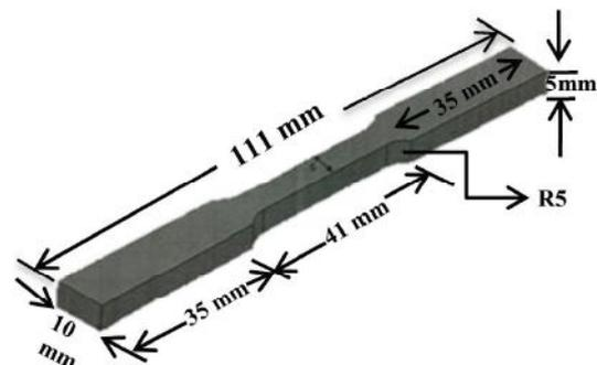
**Figure 2b Tensile Test Specimen of FSW Joint**
