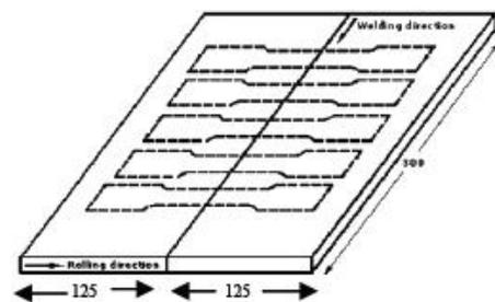
**Figure 2a Schematic Diagram Samples of FSW Joint**
