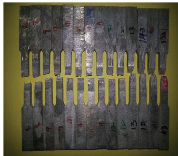
**Figure 5 Fractured specimens from Tensile Testing**
