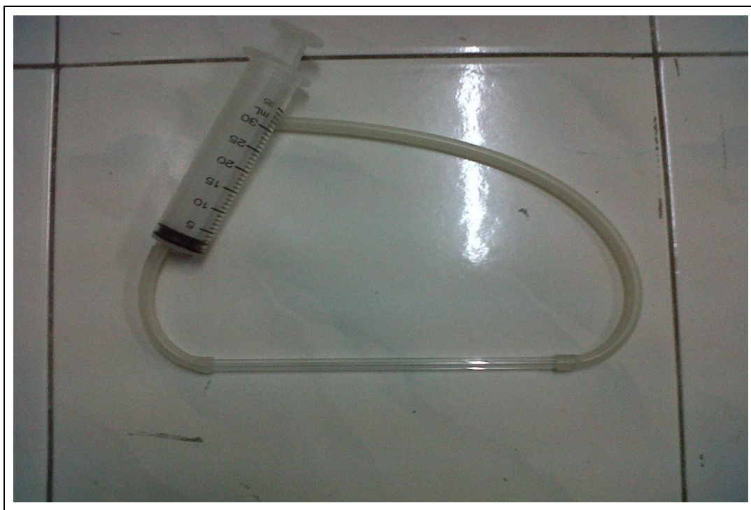
Figure 3.2: Apparatus Set-Up for Methane Gas Collection
