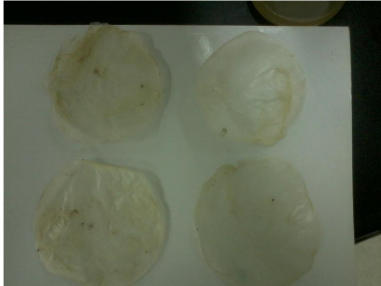
Figure A.5 Cellulose film after being treated and dried
