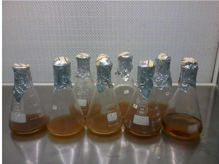
Figure A.3 PW-M was autoclaved and ready for fermentation process
