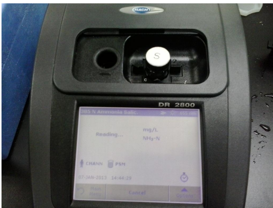
Figure C.5 Taking the ammonia-N reading for the experiment
