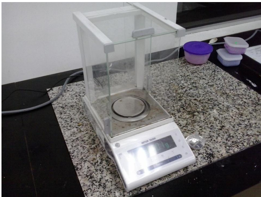
Figure C.2 Weighing balances for weight Total Suspended Solid present ( \text{NH}_3 )
