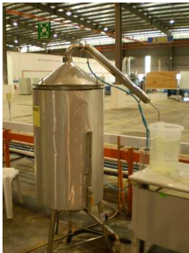
Figure 3.3: Steam Distillation Pilot Plant
