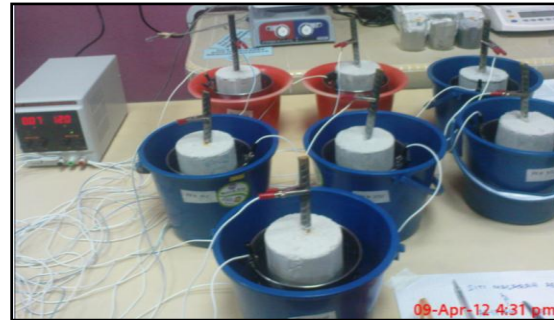
Figure 1 Accelerated corrosion test arrangement
