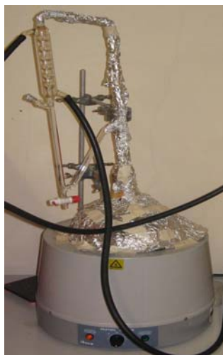
Figure 3.2: A Hydrodistillation Set-up
