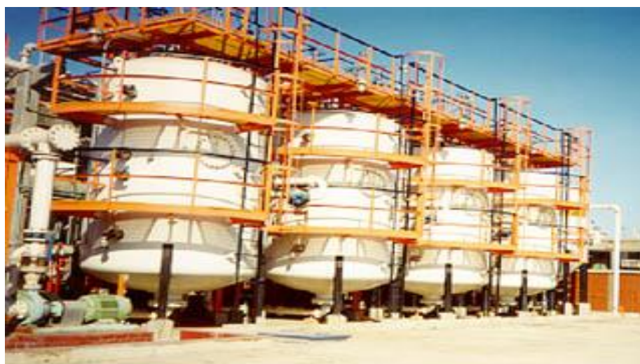
Figure 2.1 Biosorption Column Plant (B.Volesky, 2003)
