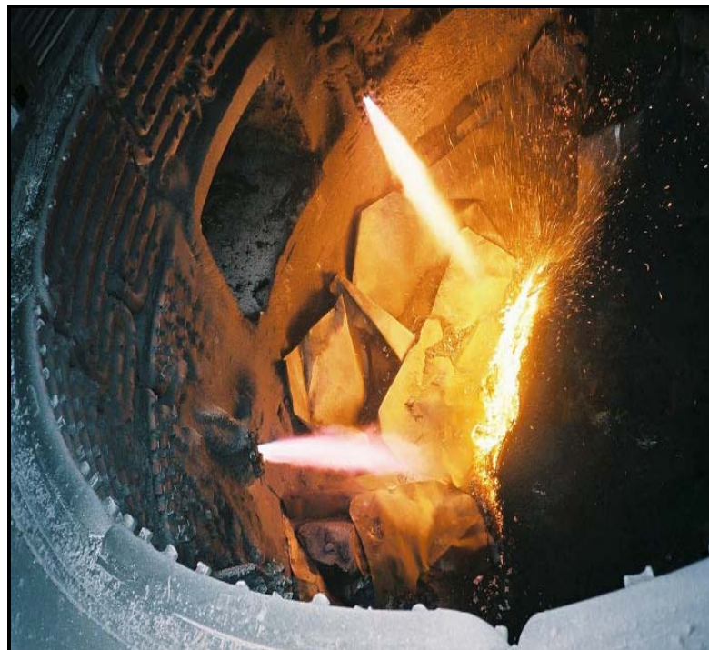
Figure 2.3: Electric Arc Furnace at PERWAJA
