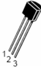
**Figure 1.10:** Typical Voltage Regulator IC
