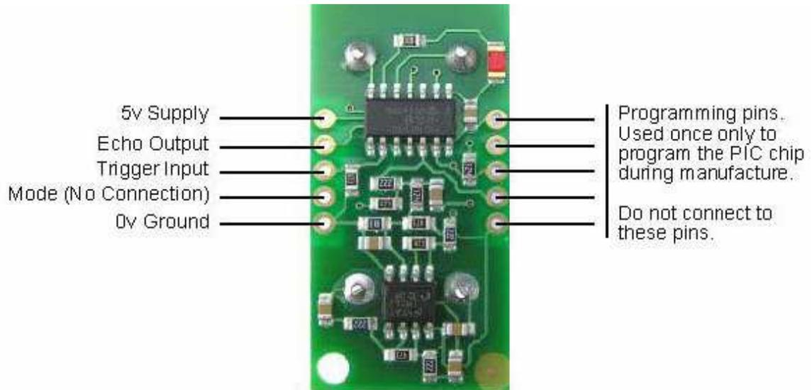
Connections for 2-pin Trigger/Echo Mode (SRF04 compatible)
