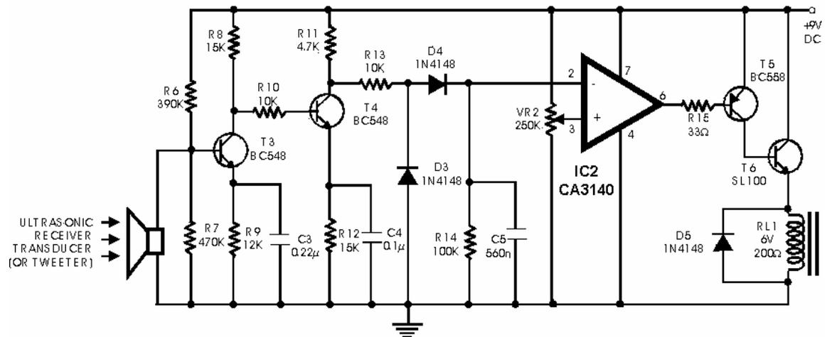
Figure 1.05: Receiver of ultrasonic sensor circuit diagram
