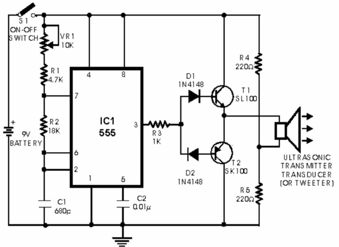
Figure 1.04: Transmitter of ultrasonic sensor circuit diagram
