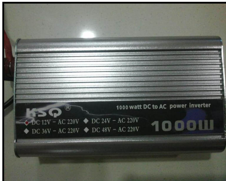
Figure 3.8: 1000 watt Power Inverter
