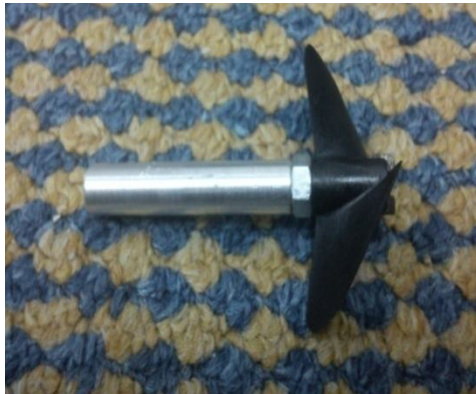
Figure 2.3: Propeller mounting to coupling shaft.
