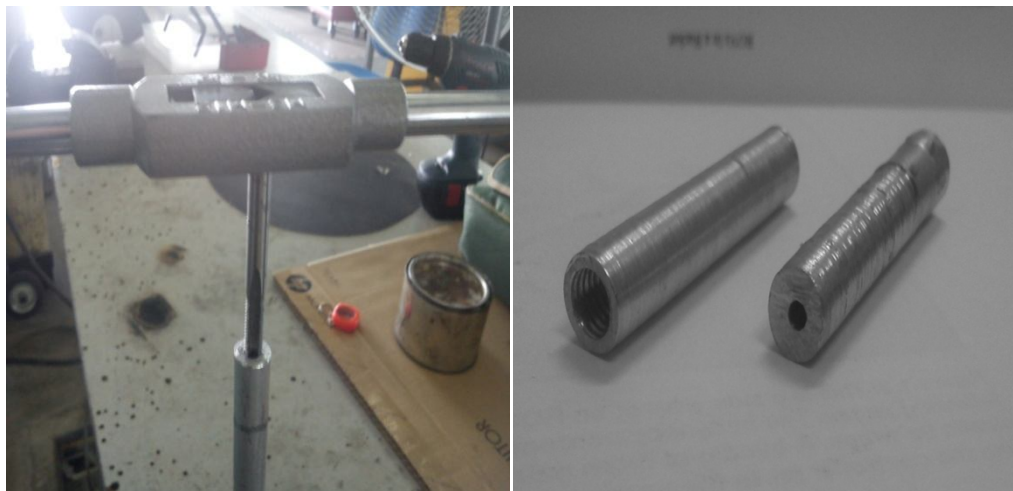
Figure 3.10 : a) Drilling process and b) the complete coupling
