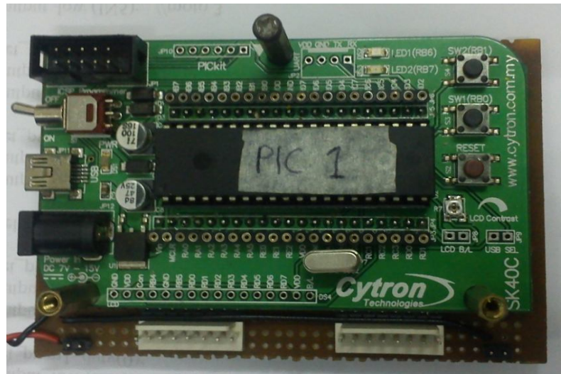
Figure 3.12 : Microcontroller circuit using Cytron circuit.
