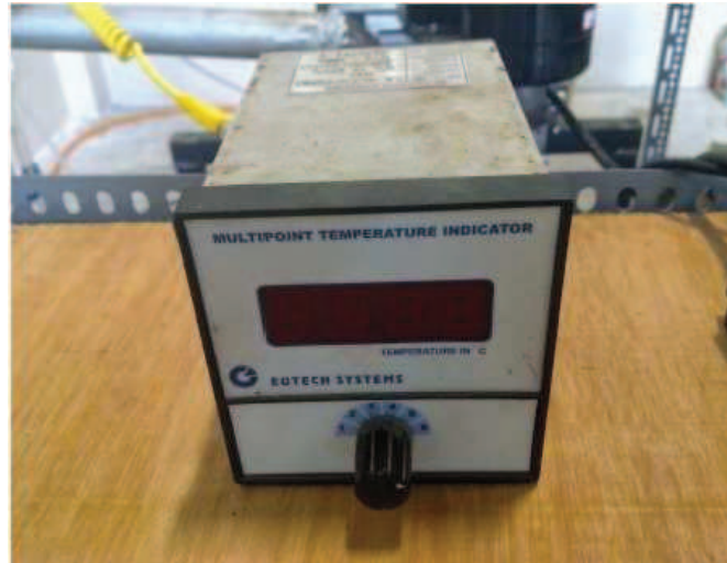
Figure 3.21: Temperature display unit
