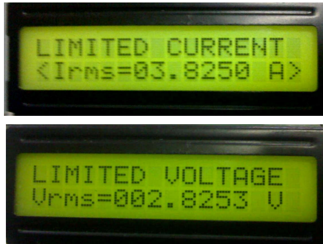
Figure 4.15: LCD shows limit voltage or current same as been display
