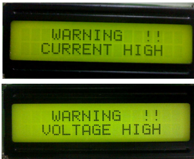
Figure 4.12: The LCD show the warning sign if current or voltage is over the limit
