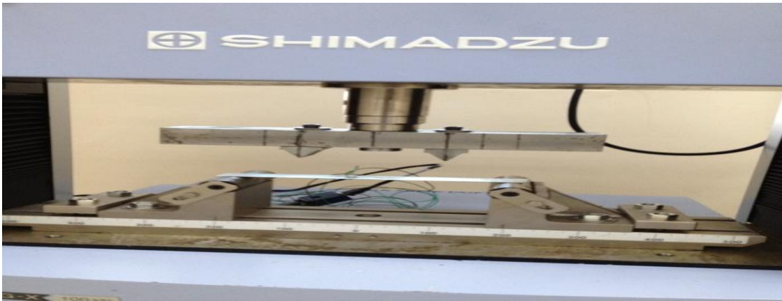
Figure 3.14: Four point bending test setup
