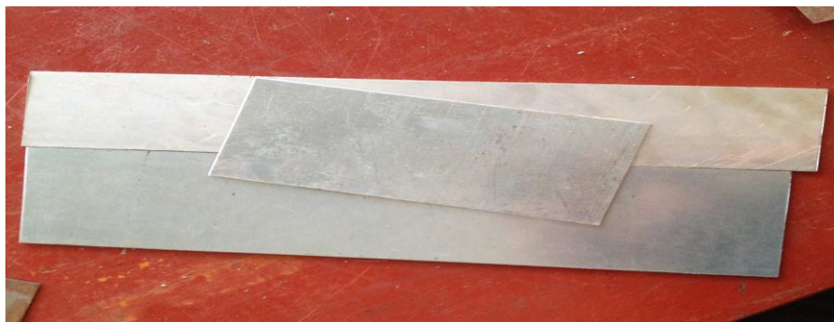
Figure 3.12: Plates of galvanized steel (220mm x 33 mm x 1mm)
