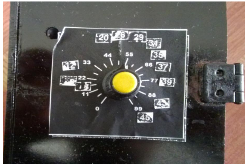
Figure 4.5: POT adjust to 52% Duty Cycle
