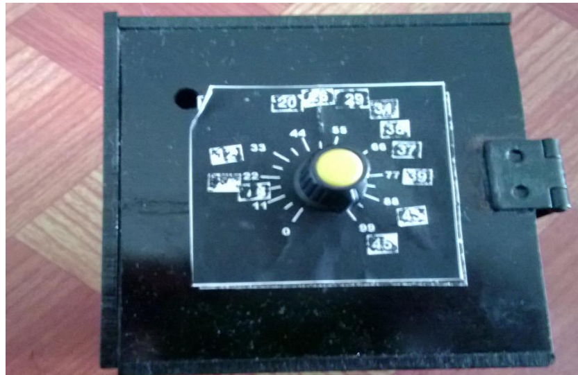
Figure 4.7: POT adjust to 99% Duty Cycle
