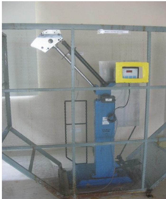
Figure 3.13: Charpy Test Machine (Digital)
